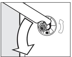
■ Using the spanner supplied, turn the left-hand transit bar 90°.
