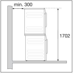
The washing machine can be installed as a washer-dryer stack together with a Miele tumble dryer. A WTV stacking kit (optional accessory) is required for this.
