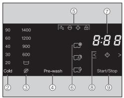
The (2, 3, 4, 6, 8) and (9) sensor controls react to fingertip contact. If a sensor control is illuminated, it can be selected.
