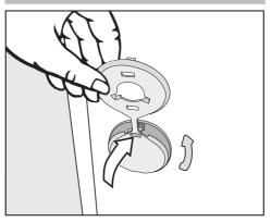
Fit the stoppers onto the two holes.
